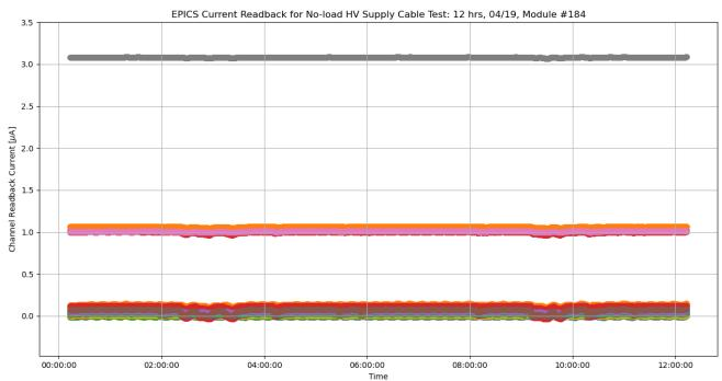
EPICS current readback data for all channels of module #184 shows one channel out of specifications
